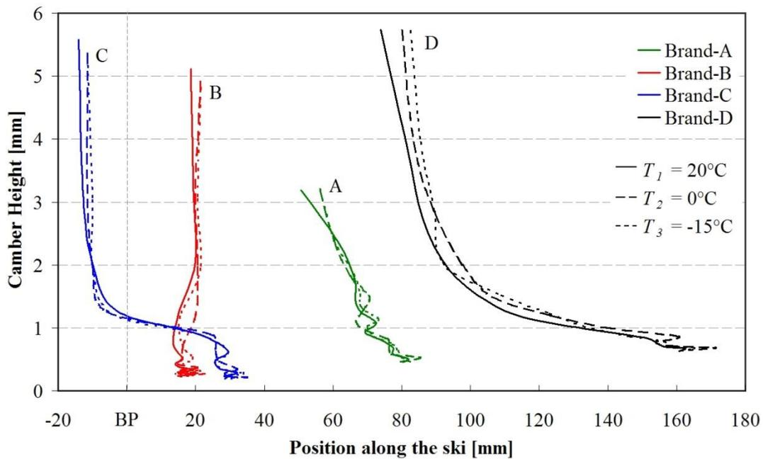
Figure A.2: The movement of the peak camber height and its location along the ski is shown for each brand (mean of both skis) and for the three different temperatures  $T_1$  (solid line),  $T_2$  (dashed line) and  $T_3$  (dotted line). The applied load increased from  $0.2$  kN to  $1.3$  kN. Just one ski was tested for brand-C.
