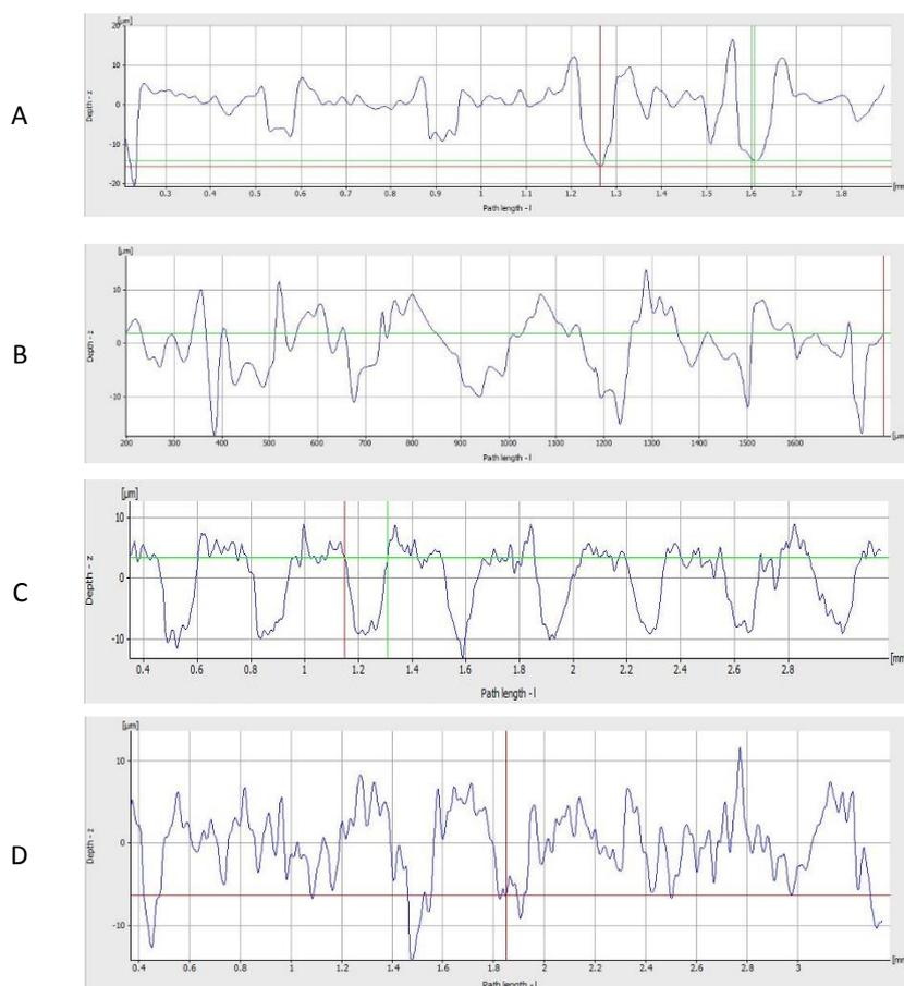
Figure 4.10: Roughness profiles from two metal cutting structures (A, B) and stone ground structures (C, D).
