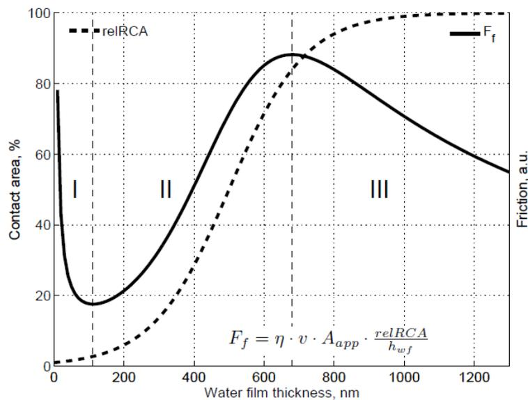
Figure 2.3: Contact area (dashed line, left axis) and friction (solid line, right axis) vs. waterfilm thickness (Bärle, 2006).
