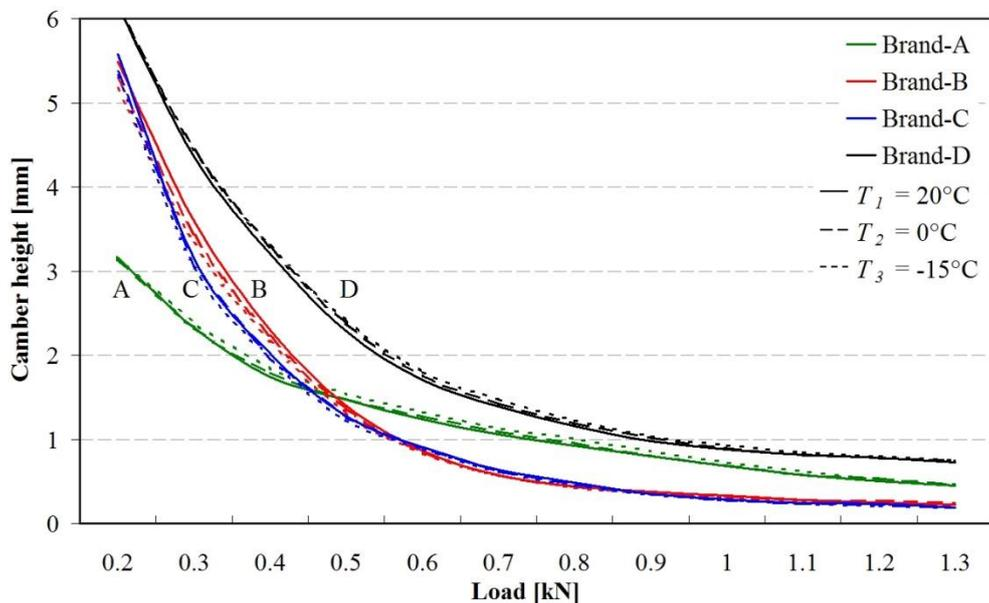
Figure A.4: Average peak Camber height for all brands at loads from 0.2 kN to 1.3 kN and the three different temperatures  $T_1$  (solid),  $T_2$  (dashed) and  $T_3$  (dotted line).
