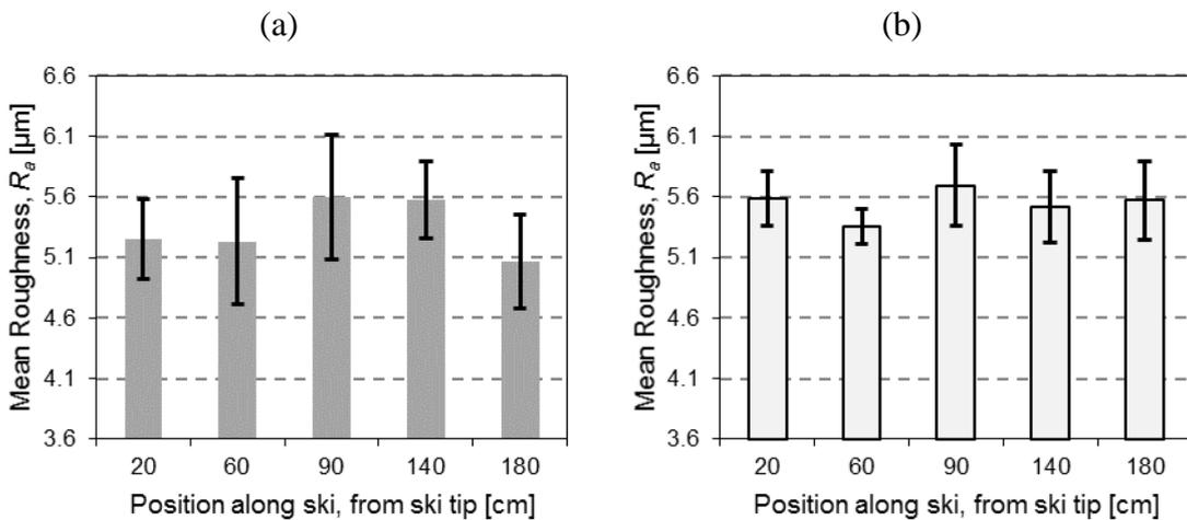
Figure G.8: Average mean roughness,  $R_a \pm \sigma$  for all five chosen measurement points along the ski; (a) stone ground skis and (b) metal ground skis.
