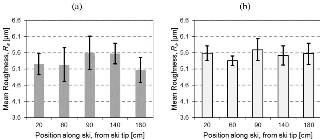
Figure 4.12: Average mean roughness,  $R_a \pm \text{SD}$  for all five chosen measurement points along the ski; (a) stone ground skis and (b) metal ground skis
