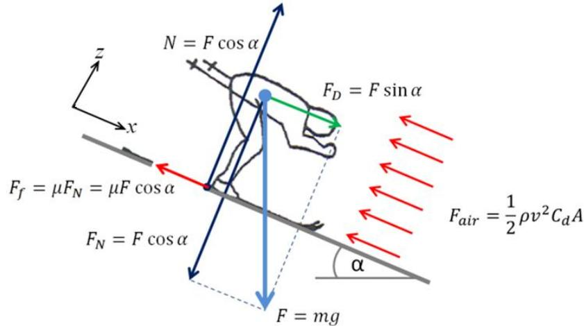
Figure 2.1: Free body diagram of forces acting on a skier in a gliding position, modified from Spring (1989).
