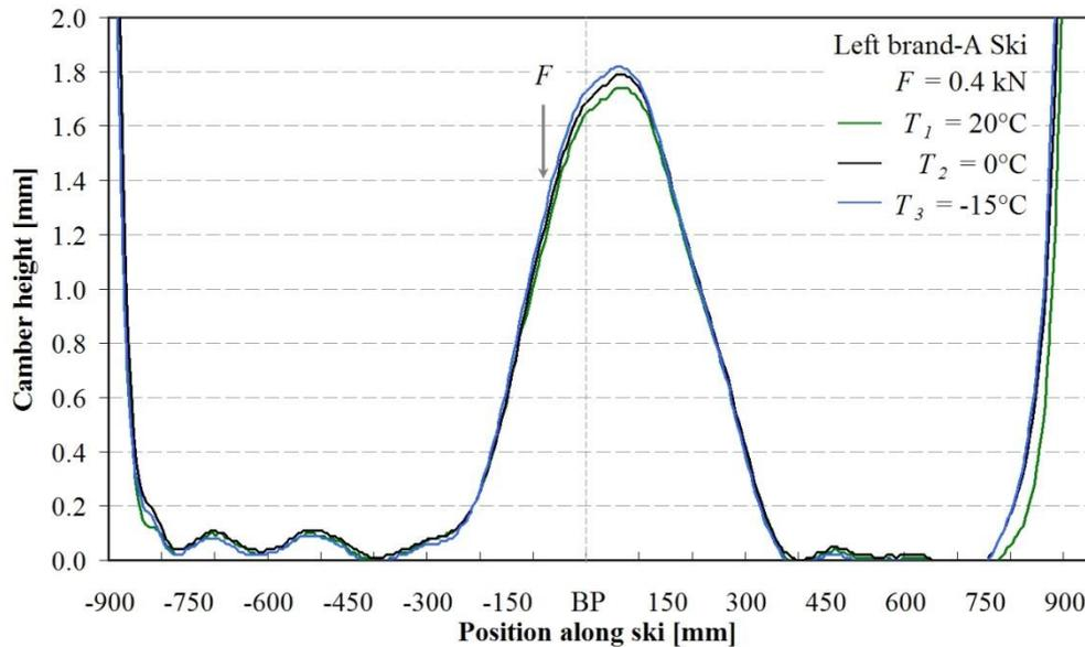
Figure A.3: Comparison of the Span-Curves for a brand-A ski loaded with 0.4 kN at three different temperatures
