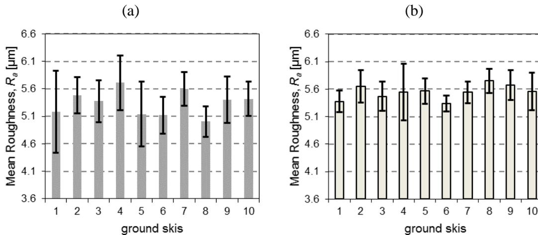
Figure 4.13: Average mean roughness,  $R_a \pm \text{SD}$  for the 10 ground skis; (a) stone ground skis and (b) metal ground skis.
