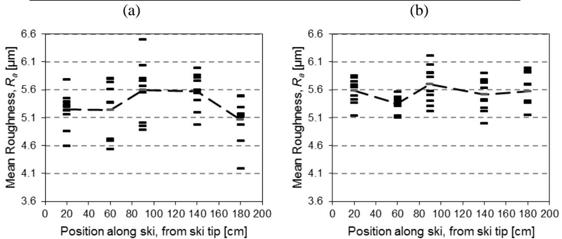
Figure 4.11: Mean roughness,  $R_a$  results for all measurement points for the five chosen points along the ski. The average of each point is connected with a dashed line; (a) stone ground skis and (b) metal ground skis.
