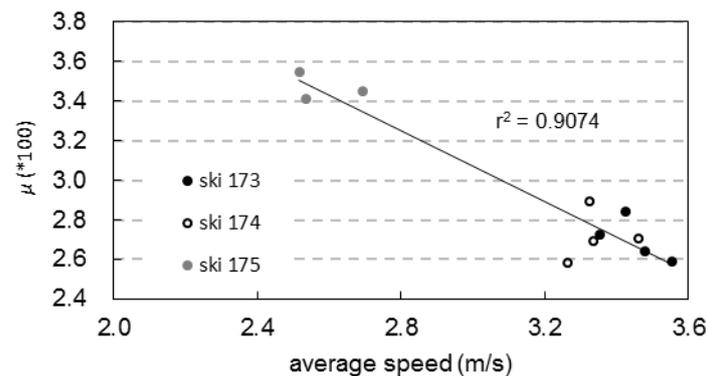
Figure 4.18: Average speed versus calculated coefficient of friction,  $\mu$  for each heat and ski with a linear regression line in black to the right.
