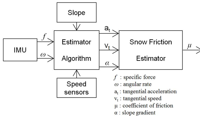
Figure 3.6: Schematic sketch of the model design for the IMU system (E).
