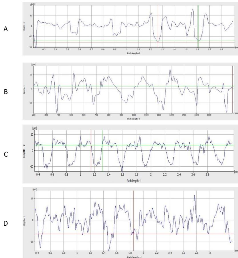
Figure G.6: Roughness profiles from metal cutting structures (A, B) and stone ground structures (C, D).
