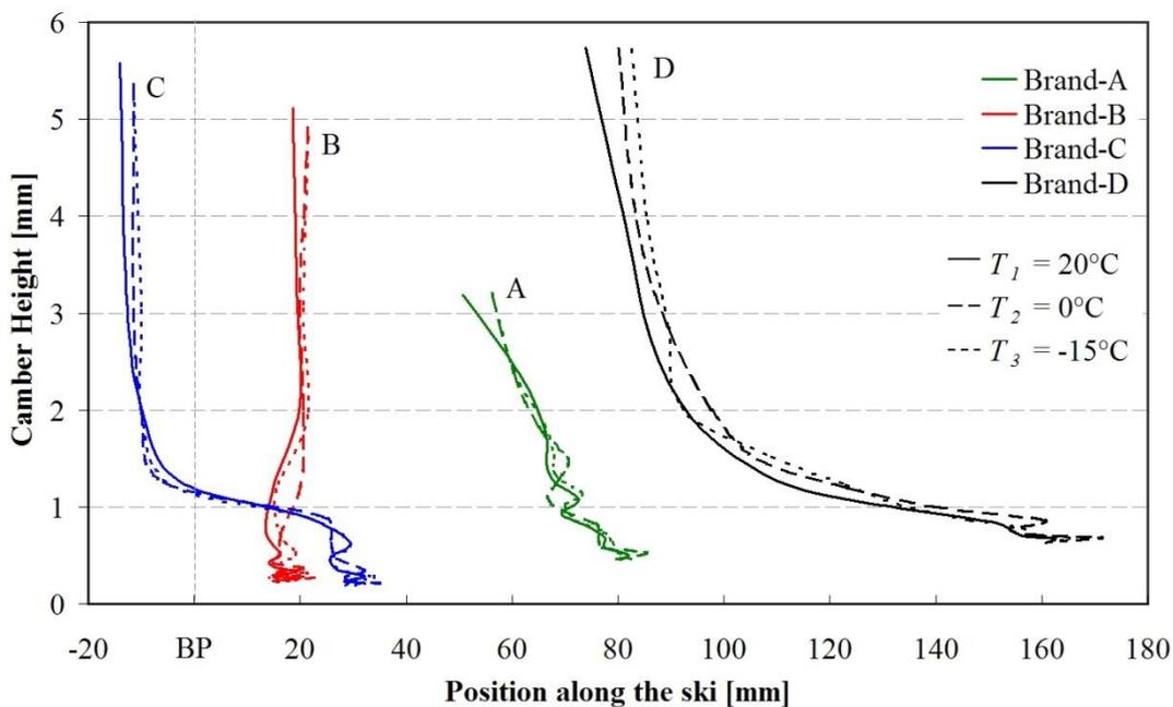
Figure 4.2: The movement of the peak camber height and its location along the ski is shown for each brand (mean of both skis), as well as for the three different temperatures  $T_1$  (solid line),  $T_2$  (dashed line) and  $T_3$  (dotted line). The applied load increased from 0.2 kN to 1.3 kN, and just one ski was tested for brand C.
