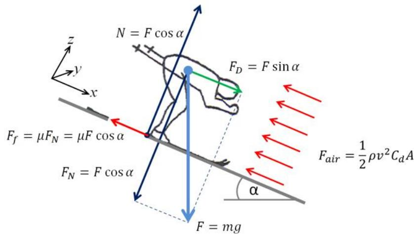
Figure E.1: Simplified forces which act on a skier in a straight downhill, modified sketch from (Spring, 1989).
