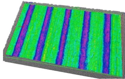
Figure 3.4: A colour-coded example of a linear stone ground structure on a ski, picture taken with an Alicona 3D microscope.
