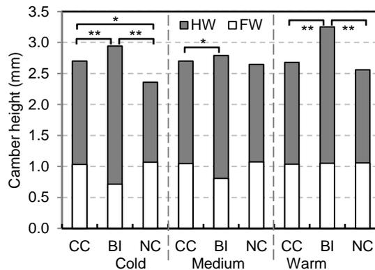
Figure C.2: Camber height at the balance point, loaded with *HBW* and *FBW* of the skiers. Significantly different between conditions at  $*P \leq 0.05$  and  $**P \leq 0.01$ .
