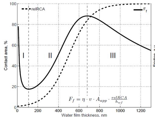
Figure G.1: Contact area (dashed line, left axis) and friction (solid line, right axis) vs. water-film thickness. Qualitative curve [11].
