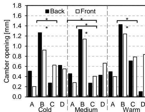
Figure 4.8: Camber opening height measured with full BW at  $\pm 41.6\%$  of the ski length in front (white) of and behind (black) the BP, with significant difference between conditions at  $*p \leq 0.05$  and  $**p \leq 0.01$ .
