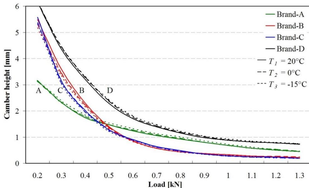
Figure 4.1: Average peak Camber height for all brands at loads from 0.2 kN to 1.3 kN and the three different temperatures  $T_1$  (solid),  $T_2$  (dashed) and  $T_3$  (dotted line).
