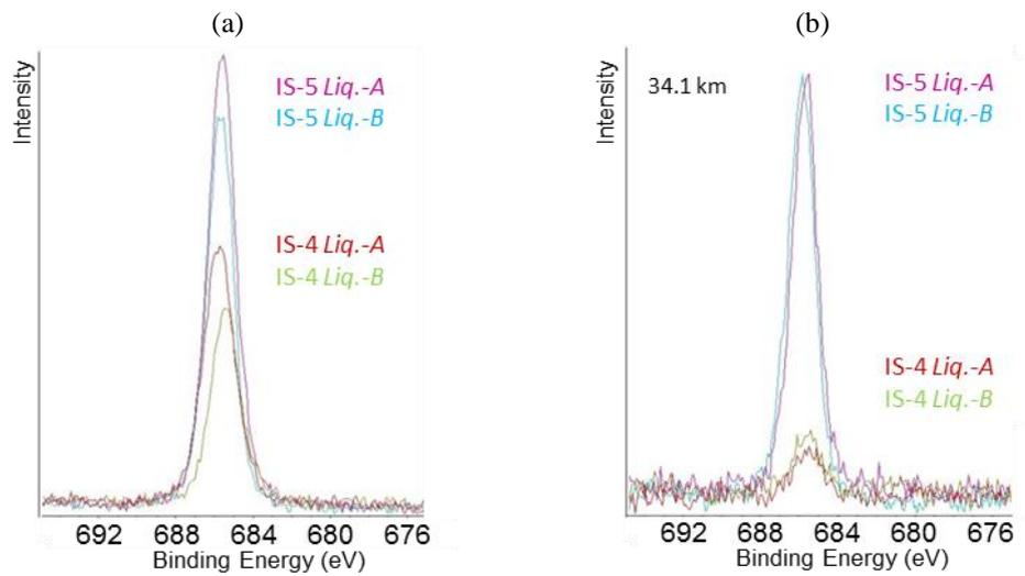
Figure 4.19: (a). XPS analyses from both base materials compared with Glider-A + Liq.-A and Liq.-B wax before skiing and (b) after skiing 34.1 km (in the spectra F 1s).
