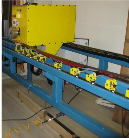
Figure G.4: Steel grinding machine with ski placed stationary in a specially designed ski bed unit and the grinding head.
