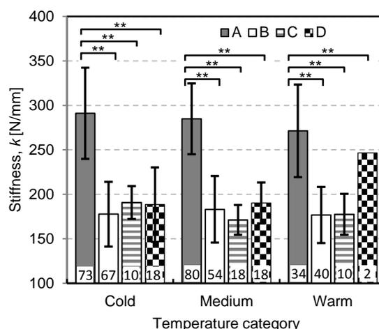
Figure 4.5: Camber stiffness,  $k$  for the four tested ski brands and all three temperature categories for male skating skis.
