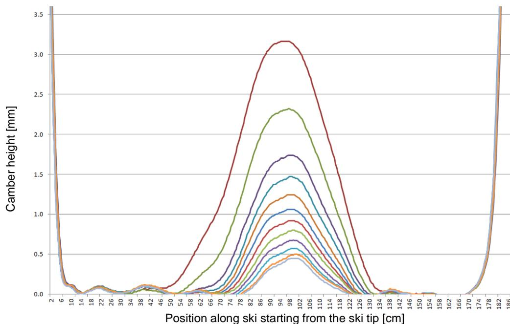
Figure 3.3: Example span curves of a classic ski loaded from 200 N to 1500 N.
