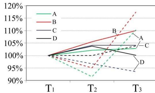
Figure A.5: Shows the early (full lines) and late (dashed lines) stiffness,  $k$  for all brands and the three different temperatures  $T_1$ ,  $T_2$  and  $T_3$ .
