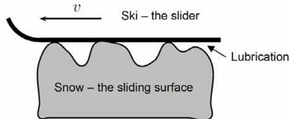
Figure 2.2: The tribological system of a ski sliding on rough snow (adapted from Bärle (2006)).
